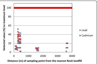
**Fig. 2** Pb and Cd results. Detected values of Pb and Cd contamination, expressed in % respect to maximum level permitted (Maximum level = 100%)
