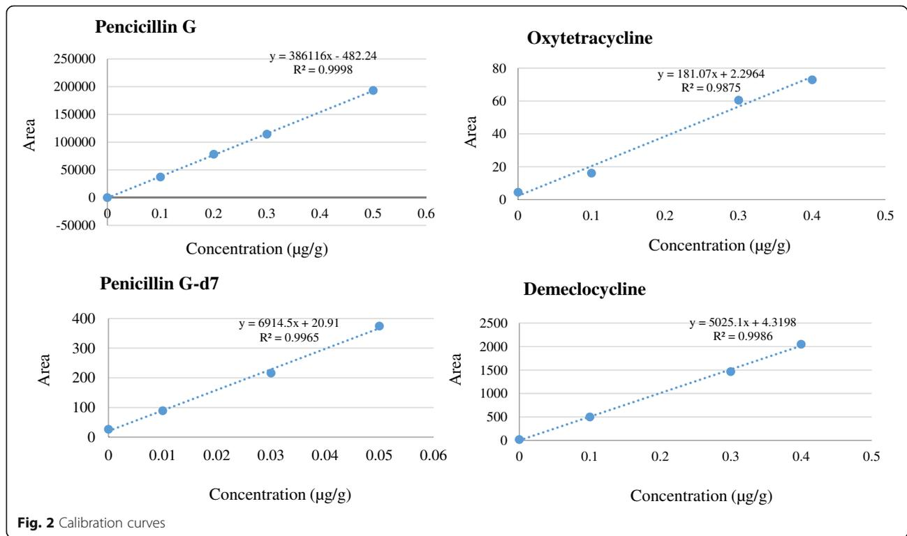
Fig. 2 Calibration curves
